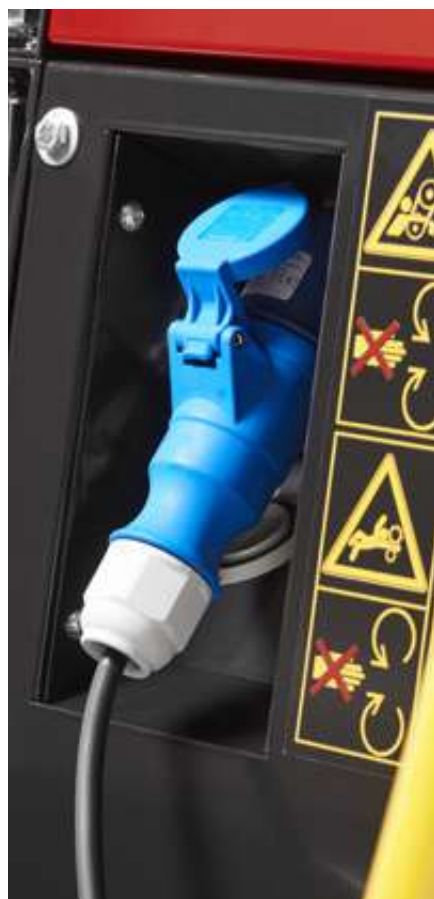
Integrated charger: 230V 16A 65V and cable
